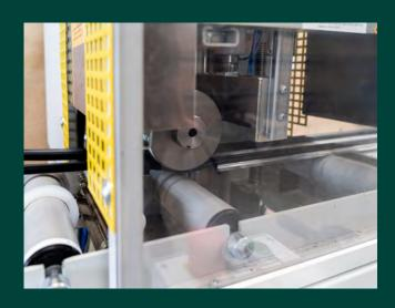
**Consistent quality:** Machine-inserted gasket ensures higher precision and consistent quality compared with manual insertion.
