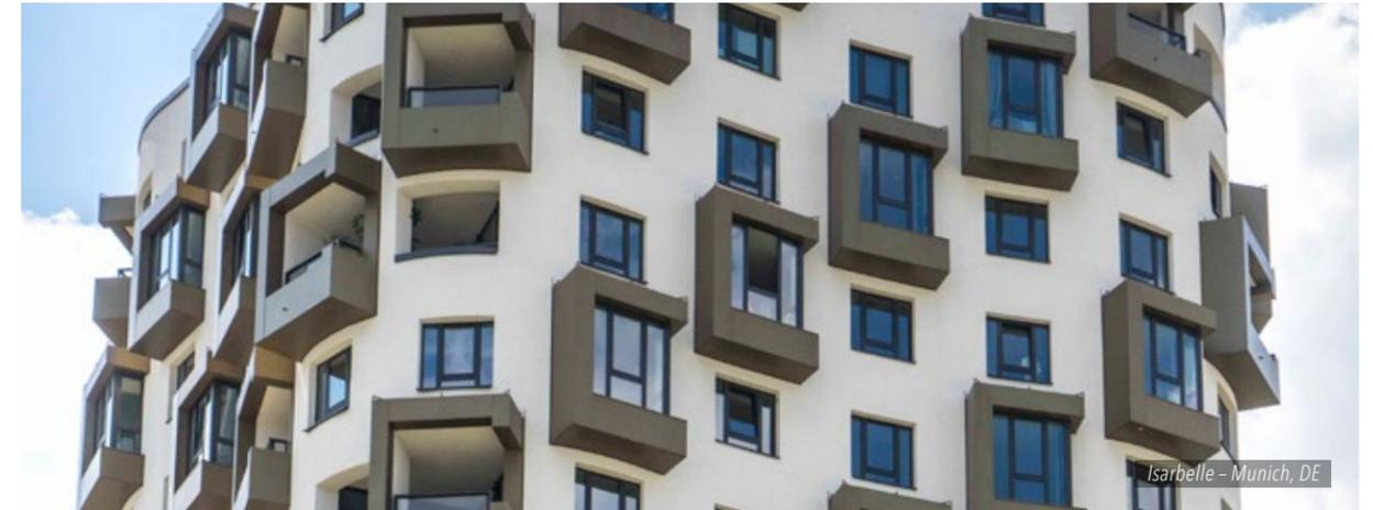
With its choice of space saving opening methods (slide to step through / tilt to provide ventilation) coupled with its outstanding thermal performance and its very high air tightness qualities, the parallel tilt and slide door is ideally suited for use as a terrace or balcony door.
