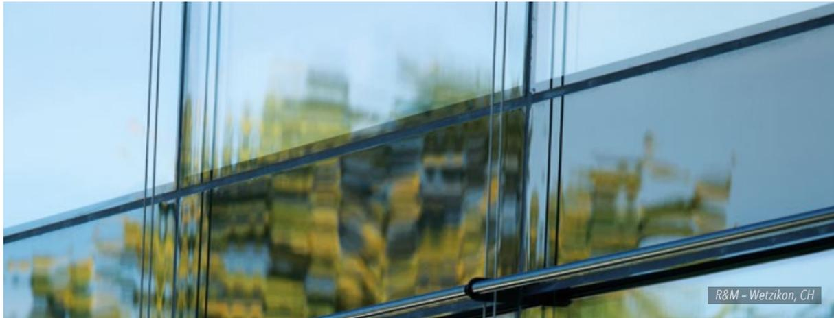
The THERM<sup>+</sup> Structural Glazing SG2 curtain wall systems feature the most intricate glazing technique. A narrow silicone joint is the only visible line between the insulation glass panes. Retention of the internal pane is enabled easily, quickly and securely with the use of SG glazing toggles. By utilising the SG insulating block, curtain walls achieve outstanding thermal insulation values.
